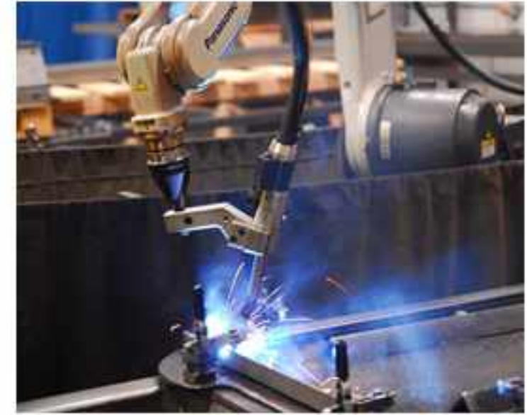
MIG WELDING/ROBOTIC (12 No.s)
