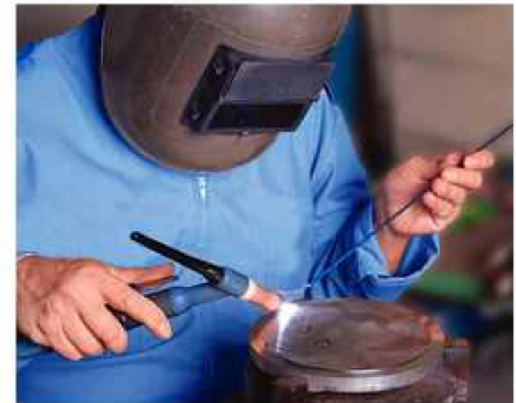
TIG WELDING (12 No.s)
